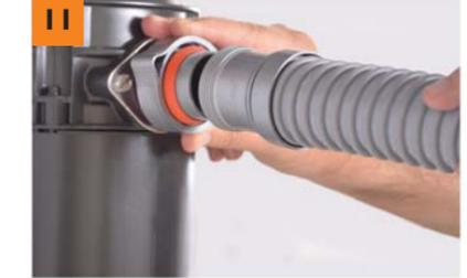
Slide slip nut (g) and an 1 1/2" orange washer (e) on tailpiece, with the conical side of washer facing out. Connect the flexible hose to the tailpiece and tighten slip nut.
