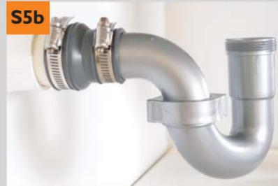
If you don't have a marvel adapter in place, use the wall coupling (d) included. (The larger side of the coupling connects to wall drains with approximately 2" exterior diameter). Insert P-Trap through coupling and into the pipe, adjust metal clamps firmly.
