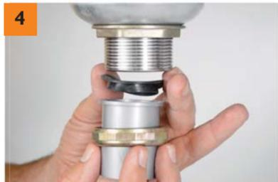
Place tailpiece washer (f) in top opening of short tailpiece (h), and slide strainer locknut from the bottom. Insert tailpiece into strainer and tighten locknut.
