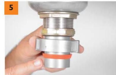
Slide slip nut (g) and a 1 1/2" orange washer (e) in short tailpiece, with conical side of washer facing down.
