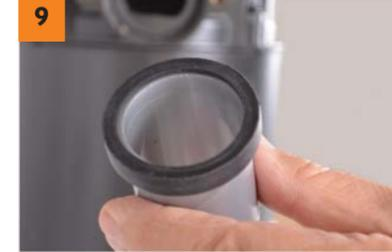
Locate the black washer included in your disposal parts. There is a groove in the washer that fits over tailpiece lip. Place washer over lip. (The flat side of washer facing disposal outlet).
